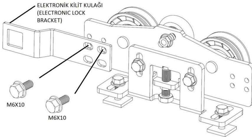
Assemble to the carrier pulley the electronic lock bracket with 2 M6x10 flanged bolts.
