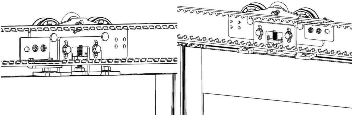
**IMPORTANT NOTE :** When attaching the belt to the belt bracket, always align the bracket with the center of the left belt bracket.
