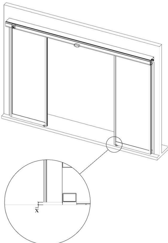
x value must be between 12 mm and 15 mm.
