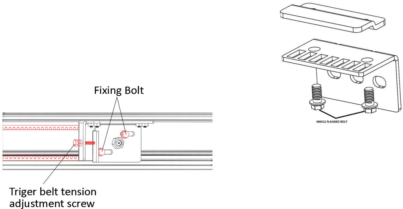
Arrange the belt tension with belt adjusting bolt.
