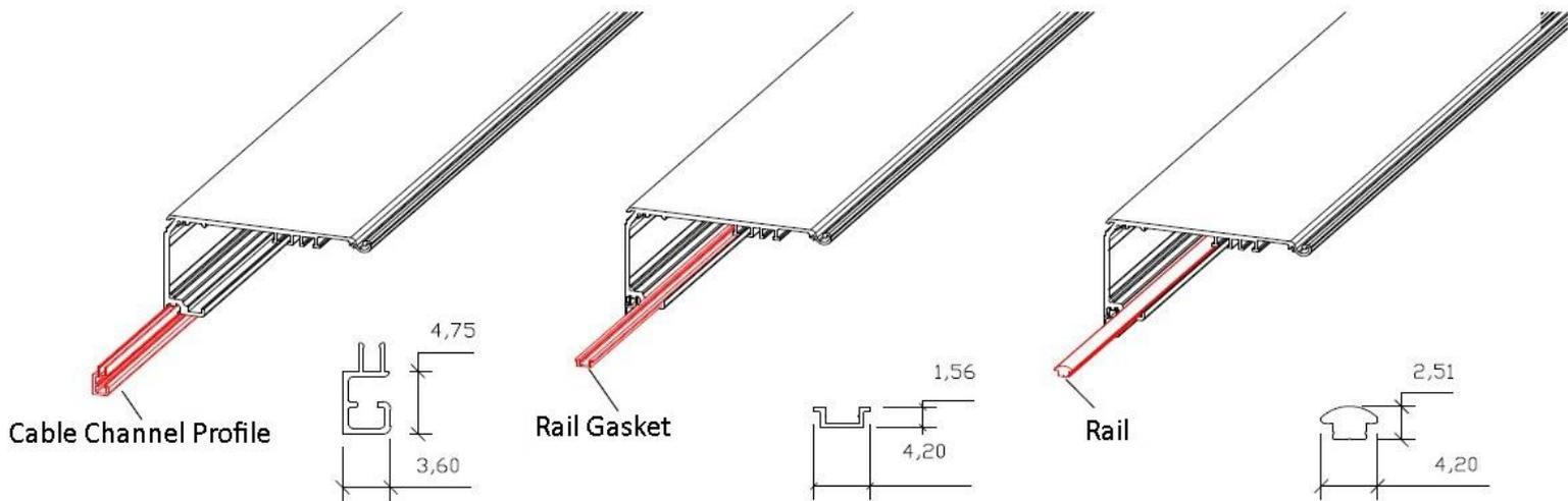
**Place the cable channel profile to the fixture/chassis passage.**
