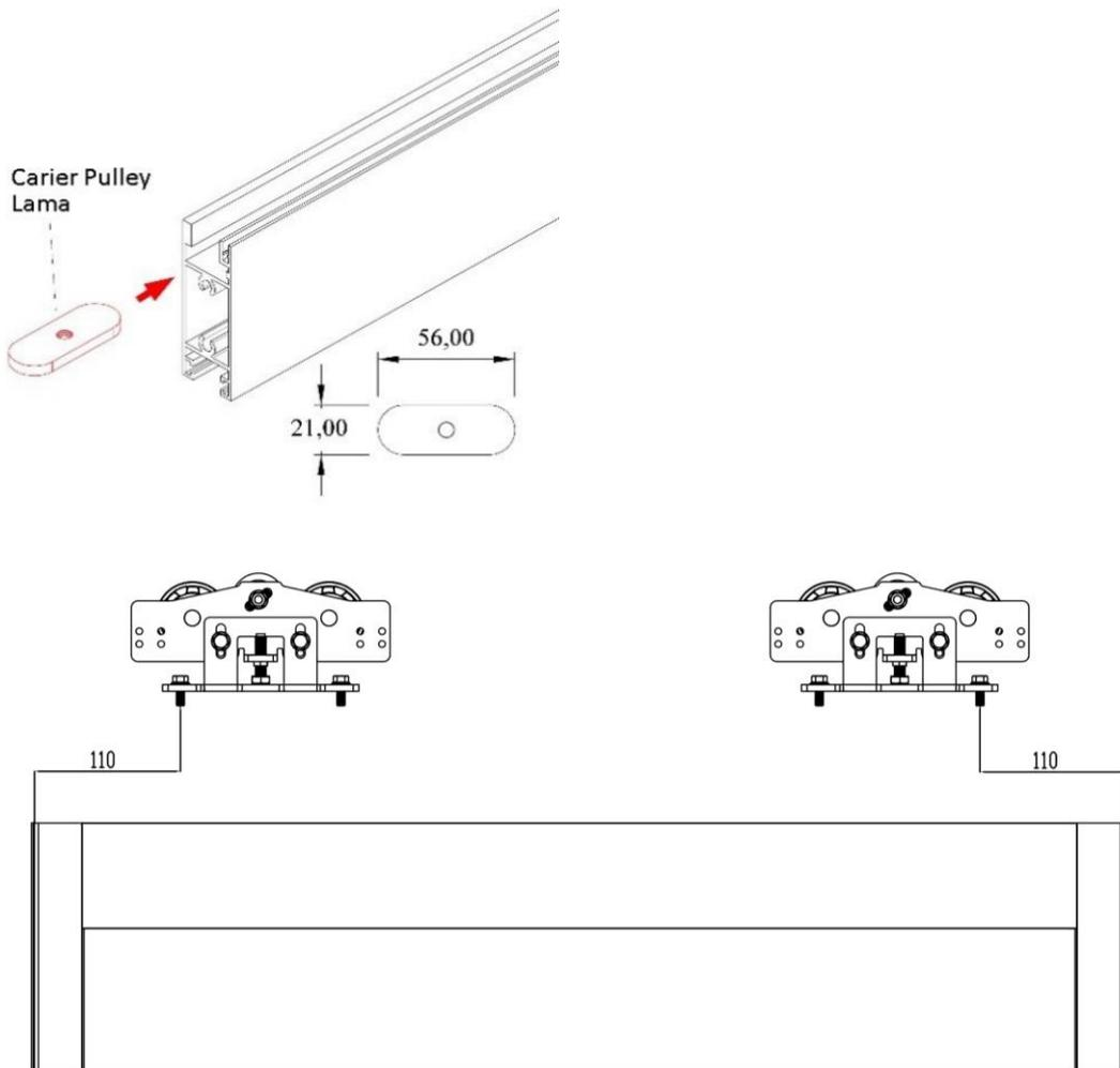
The carrier pulley are secured with bolts M6x22 flange bolted to the Lama which is positioned so that the horizontal profile is 110 mm away from the joints. In some cases the distance may be reduced or increased.
