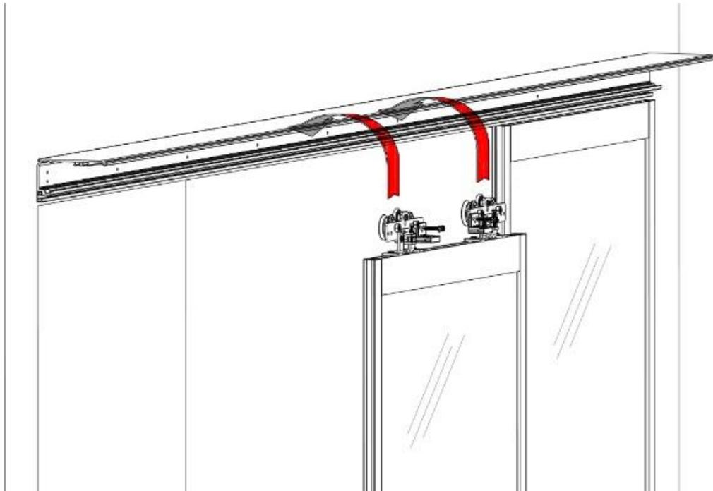
Once the leaf has been collected after mount it on chassis. The height adjustment is made so that a distance of 1 mm is maintained between the carrier pulley balance roller and the mechanism.
