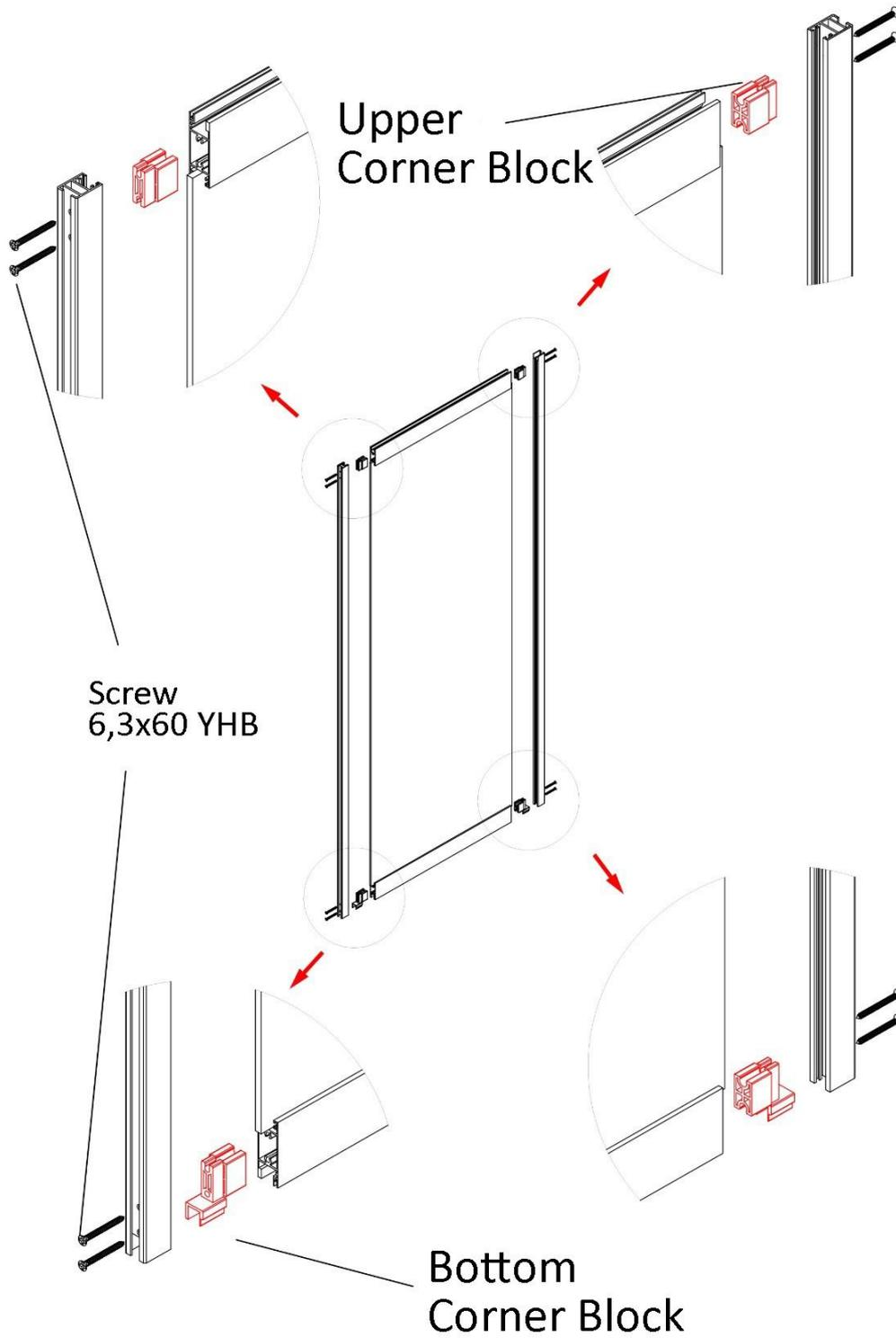
First, the upper horizontal profile is inserted into the 4 plates to hold the carrier pulley. Vertical profile horizontal profile After the glass is placed as shown fixed with 6.3x60 corner pick screw. Once the leaf has been collected, the glass seal, front and rear mating seals are placed according to the details on page 27.
