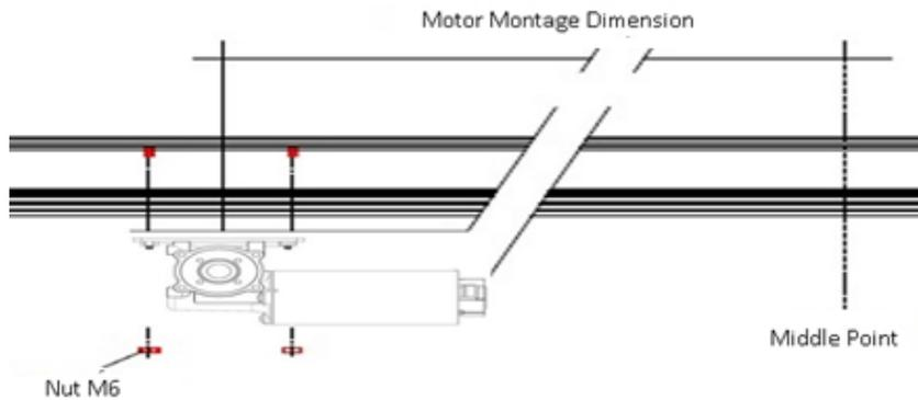
**By right side opened doors ; assemble the motor in the following dimension = 20 cm from the left edge.**
