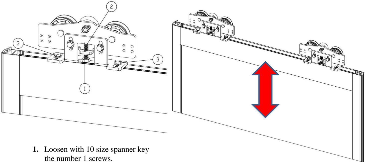
1. Loosen with 10 size spanner key the number 1 screws.
