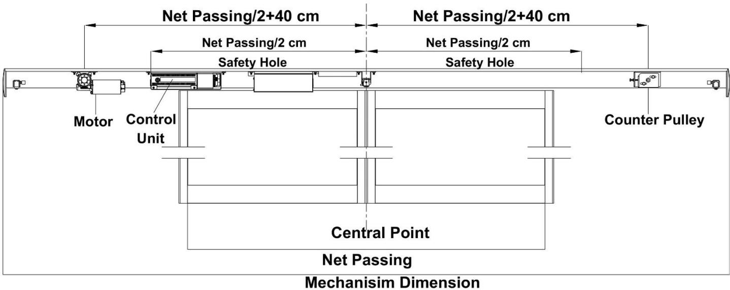
1. During preparation of mechanism, first find center (midpoint)
