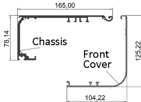
**1- Place the bended part at the top of the front cover into the groove on the Fixture/chassis.**
